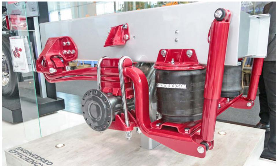
Hendrickson is its COMFORT AIR, serial production of which commenced in India last October for an OEM in the domestic e-bus market. “The COMFORT AIR is our solution tailor-made for electric buses. The purpose of offering it for e-buses is because e-buses require a battery space and to create the required level of balancing and stability, the market is not very comfortable with the cow horn design which is why this particular design has been made”, he reveals.
