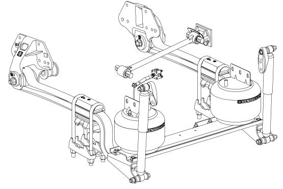
The COMFORT AIR rear air suspension system for applicable Lion Electric Buses delivers an innovative suspension solution for an electric bus. The system combines superior comfort, outstanding ride, improved handling, and reduced maintenance.
