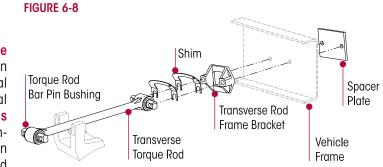
and/or the torque rod bushings will require replacement if any of these conditions are encountered.
