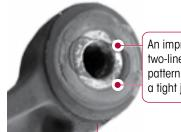
An imprinted two-line wear pattern exhibits a tight joint
