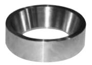
These shop made tools are designed to install and remove torque rod bushings. Bushing tools are made from cold rolled steel or equivalent. Drawings are for reference only. Hendrickson does not supply these tools.
