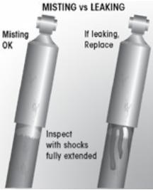
Inspect the shock absorber fully extended. A shock absorber that is truly leaking will show signs of fluid leaking in streams from the upper seal, see Figure 6-11. These streams can easily be seen, underneath the main body (dust cover) of the shock absorber. Replace as necessary.
