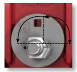
Maximum range of adjustment is  $\pm$  90 degrees from 12 o'clock position.
