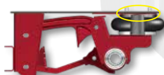
Figure A: Primary (airbag) bump stop engages
