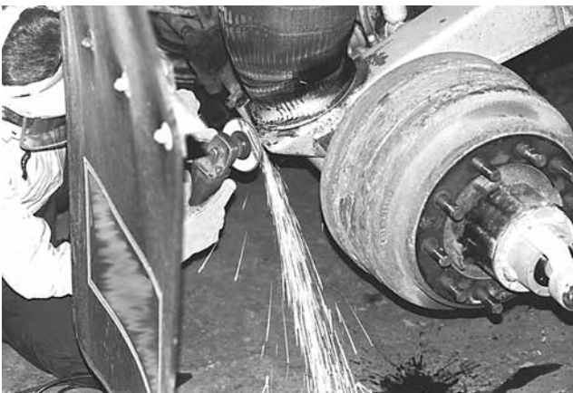
Figure 68: Preparing rear suspension beam ends
