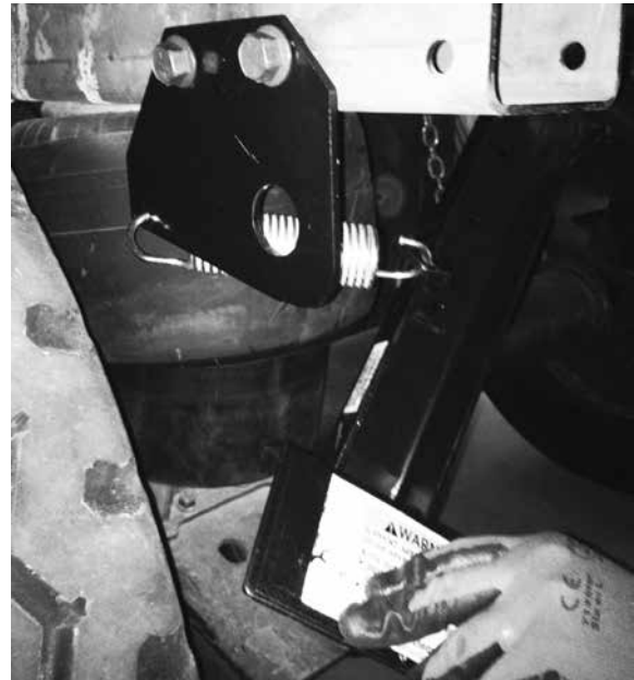
Figure 21: Arm raised above rail for spring installation
