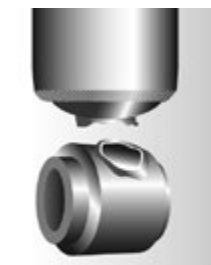
Damaged upper or lower mount
