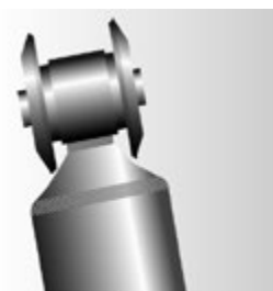
Improper installation Example: washers (if equipped) installed backwards.
