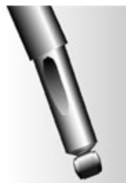
Bent or dented shock
