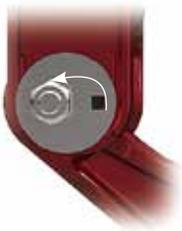
QUIK-ALIGN — Rotating the eccentric collar allows up to 1-inch of axle alignment per side
