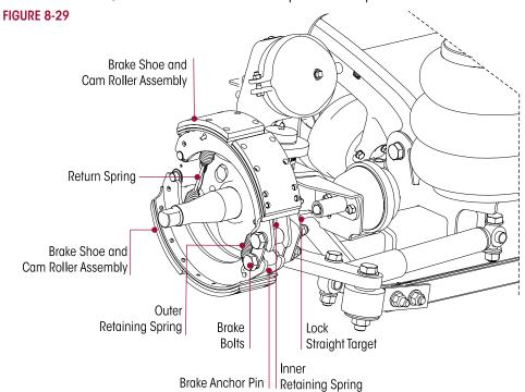
5. Remove the outer retaining spring and inner retaining spring (See Figure 8-30).
