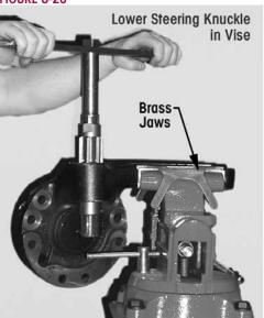
**FIGURE 8-21** Upper Steering Knuckle in Vise **Brass Jaws**
