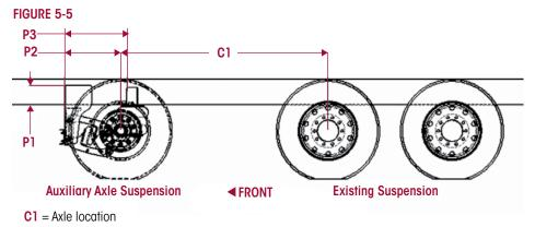
P1, P2, P3 = Dimensions located on Hendrickson suspension assembly drawing provided in your parts box.
