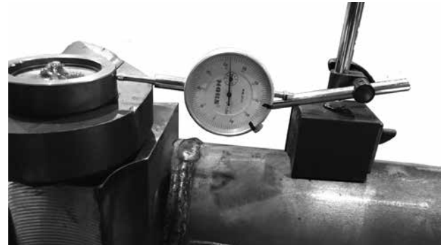
Figure 18: Checking upper kingpin bushing
