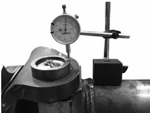
Figure 31: Checking steering knuckle vertical end play
