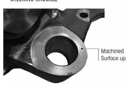
Lay the kingpin seal into the bore of the steering knuckle. The lip should face outward, toward the axle.
