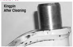
2. Inspect the kingpin for wear or damage. Use a micrometer and measure the upper and lower kingpin in two locations. Positions must be 90° opposed from each other. If the kingpin has less than 1.802" diameter, replacement of the axle is necessary, see Figures 9-54 through 9-57. Kingpin minimum dimension is 1.802".
