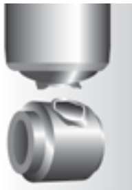
Damaged upper or lower mount
