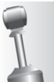
Damaged dust cover and / or shock body
