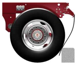
Pivoting mud flap brackets are more effective at preventing component damage than traditional brackets. If the mud flap is pinched between the tire and an obstacle behind the trailer, the entire bracket can rotate in the same direction as the flap is being pulled.
