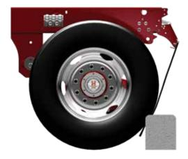
Tension is evenly distributed along the top of the mud flap as the brackets rotate downward, protecting the outermost edges of the mud flap from being torn. Since the brackets are springloaded, once the mud flaps are no longer pinched and pulled, the brackets return everything back into place undamaged and ready for continued operation.
