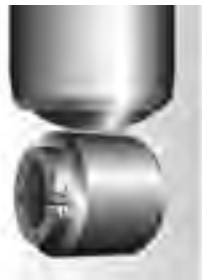
Damaged upper or lower bushing
