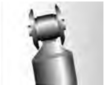
Improper installation Example: washer (if equipped installed backwards)
