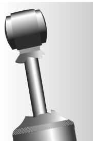
Damaged dust cover and / or shock body
