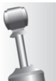
Damaged dust cover and / or shock body
