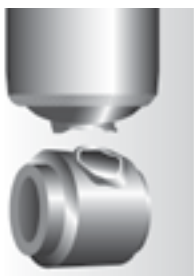
Damaged upper or lower mount
