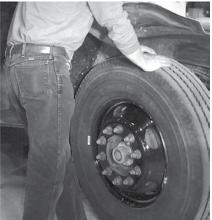
9. Move the bottom of the tire in and out. If the dial indicator moves more than 0.015", the lower bushing is worn or damaged. Replace both kingpin bushings. Refer to the Component Replacement section in this publication.
