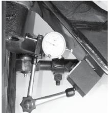
FIGURE 7-18 Move the TOP and BOTTOM of the tire in and out
