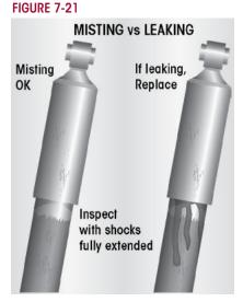
Inspect the shock absorber fully extended. A shock absorber that is truly leaking will show signs of fluid leak-
