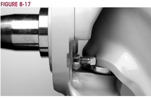
7. Measure the wheel cut and check for any interference with related steering components.
