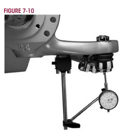
According to the Commercial Vehicle Safety Alliance (CVSA), the "out of service" criteria for front steer axle tie rod assemblies on any commercial vehicle is: Any motion other than rotational between any linkage member and its attachment point of more than 1/8" (3 mm) measured with hand pressure only. (393.209(d)), (published in the North American Standard Out-of-Service Criteria Handbook, 2022.)
