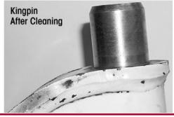
Inspect the kingpin for wear or damage. Use a micrometer and measure the upper and lower kingpin in two locations. Positions must be 90° opposed from each other. If the kingpin has less than 1.802" diameter, replacement of the axle is necessary, see Figures 9-37 through 9-40. Kingpin minimum dimension is 1.802".
