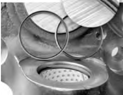
FIGURE 9 Magnification of lip seal Lip seal faces toward axle
