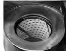
FIGURE 11 STEERTEK Magnification of the kingpin bushing and a SINGLE lip seal installed in the steering knuckle.
