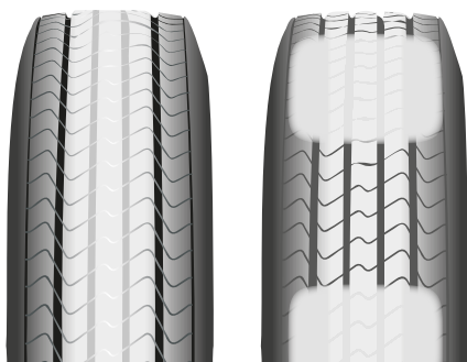
Figure 218: Centre Wear & Flat Spot Tyre Wear Patterns
