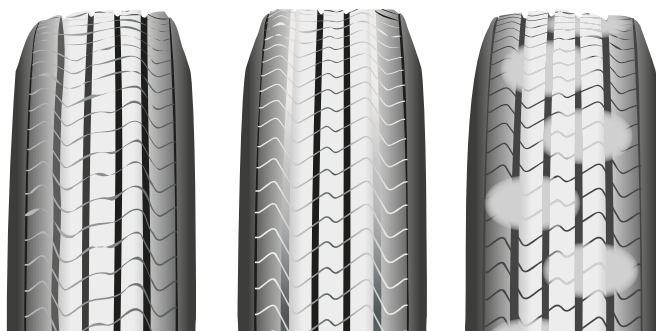
Figure 219: Feathered, Edge Wear, Cupped Wear Patterns
