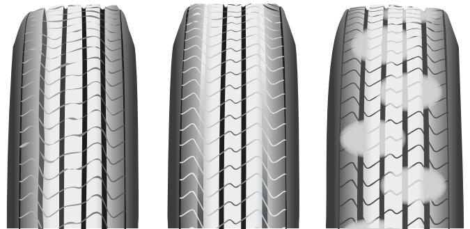
Figure 219: Feathered, Edge Wear, Cupped Wear Patterns
