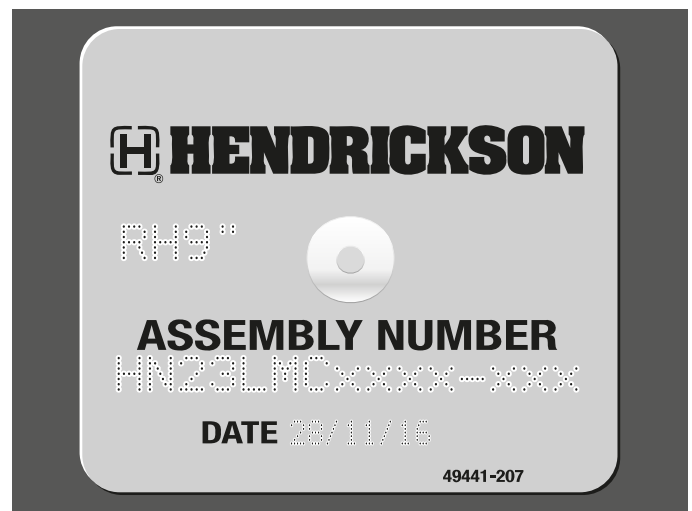
Figure 16: Axle Assembly Number Plate
