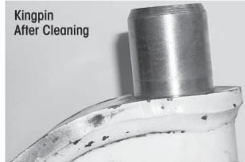
2. Inspect the kingpin for wear or damage. Use a micrometer and measure the upper and lower kingpin in two locations. Positions must be 90° opposed from each other. If the kingpin has less than 1.802" diameter, replacement of the axle is necessary, see Figures 9-7 through 9-10.
