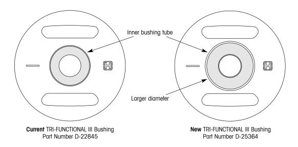
We also increased the stiffness of the new TRI-FUNCTIONAL III Bushing, making it more durable than the current bushing. Because of the increased stiffness and durability, the new and current bushings will wear unevenly if used on the same axle. Therefore, the new TRI-FUNCTIONAL III Bushing and the current bushing must not be mixed on the same axle. The new TRI-FUNCTIONAL III Bushings in this kit must be installed in both suspension pivot connections.
