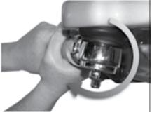
Push up and down in a push-pull motion to check any movement or looseness
