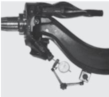
FIGURE 7-5 Move the TOP and BOTTOM of the tire in and out
