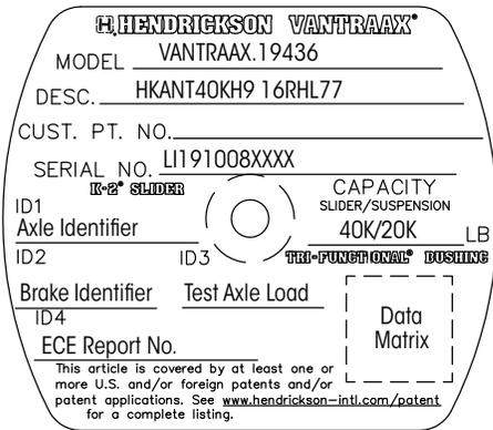
For sliders, located roadside front, on slider rail above frame bracket or on frame bracket. For HT™ Series Suspensions and INTRAAX® Integrated Air Suspension Systems, located inward side of either curbside or roadside suspension beam.
