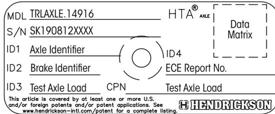
Located on leg of (air) brake chamber bracket, either on outboard or inboard side.
