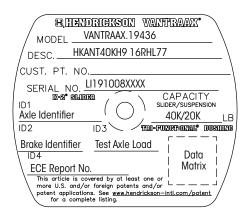
For sliders, located roadside front, on slider rail above frame bracket or on frame bracket. For HT<sup>TM</sup> Series Suspensions and INTRAAX® Integrated Air Suspension Systems, located inward side of either curbside or roadside suspension beam.
