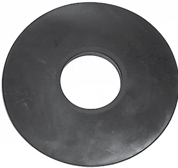
Normal bushing tube spacer in serviceable condition.
