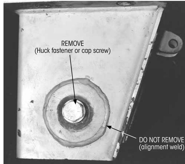
Figure 8: Removing welded collar pivot bolt
