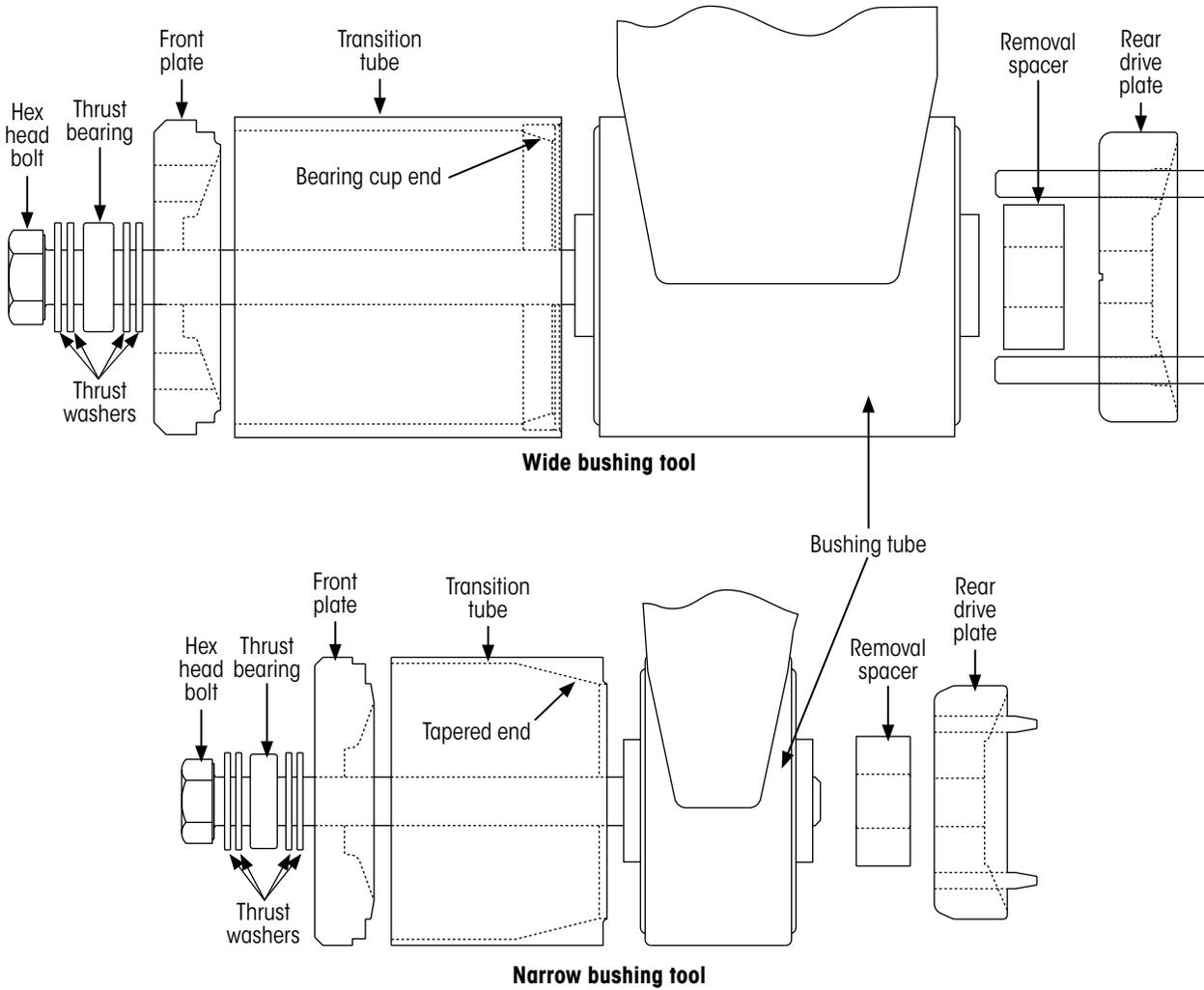
Figure 17: Assembling bushing tool for removal
