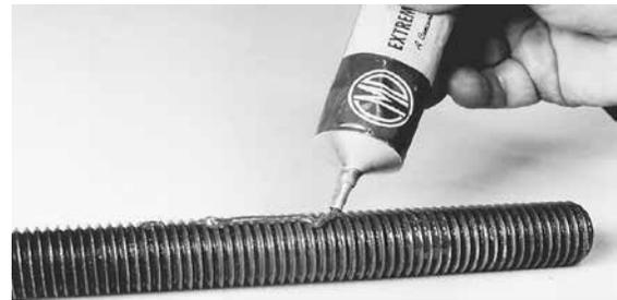
Figure 15: Applying lube to the hex head bolt
