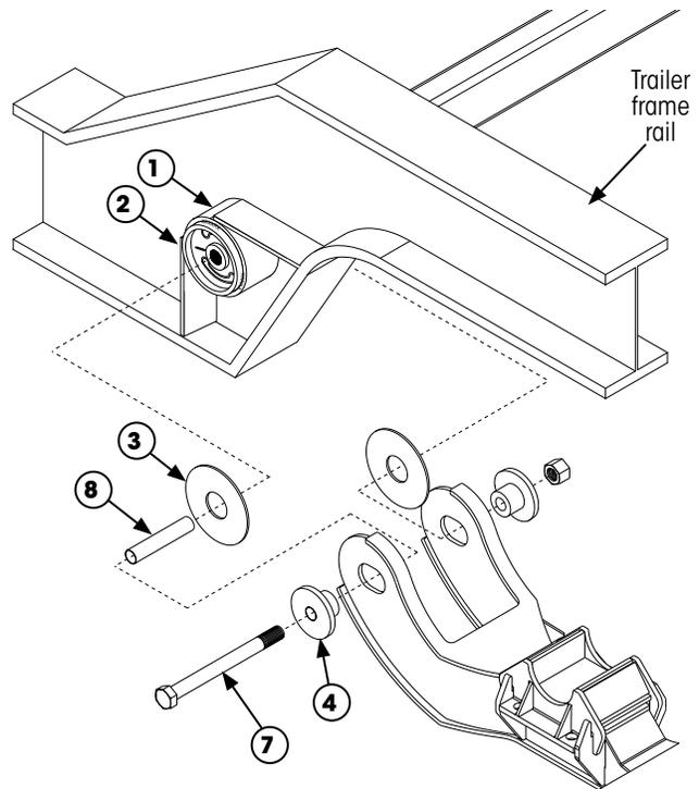
Figure 49: Welded collar pivot connection hardware
