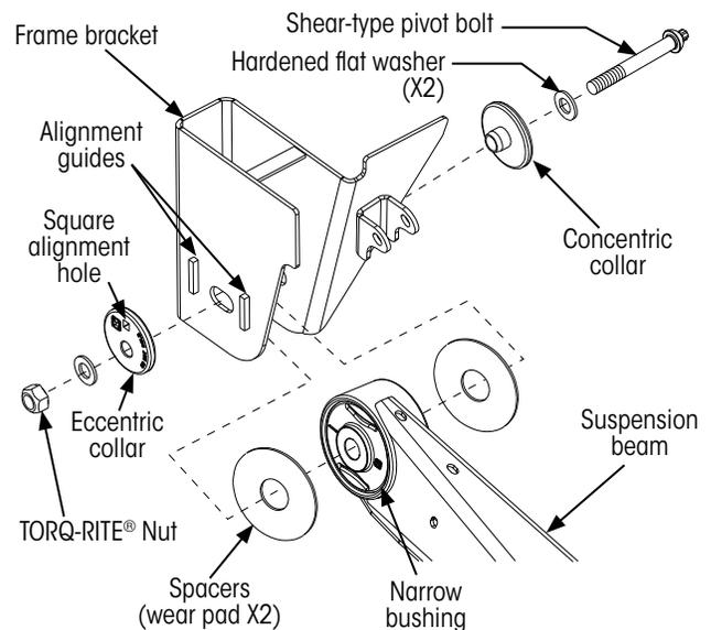
Figure 5: QUIK-ALIGN style pivot connection hardware (narrow bushing shown)
