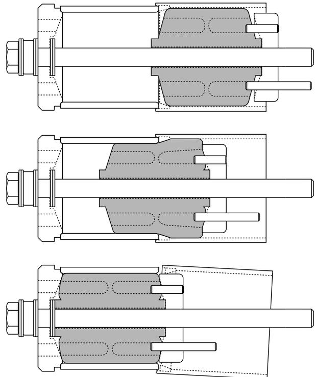
Figure 45: Typical bushing installation progression as hex head bolt is turned
