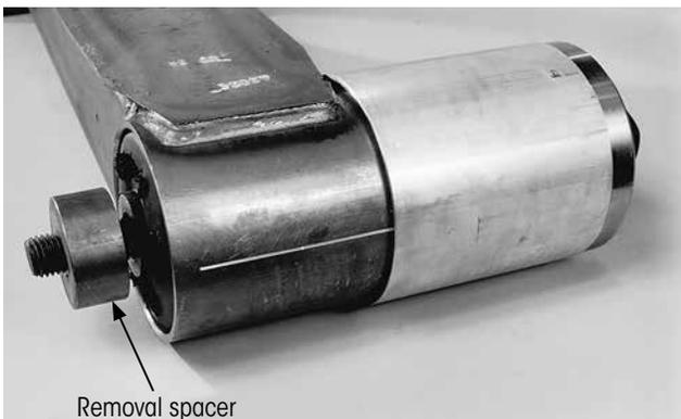
Figure 20: Installing removal spacer
