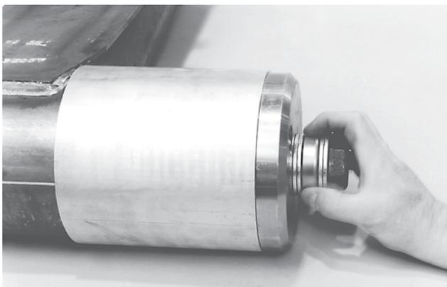
Figure 25: Ensure thrust bearing is free to turn
