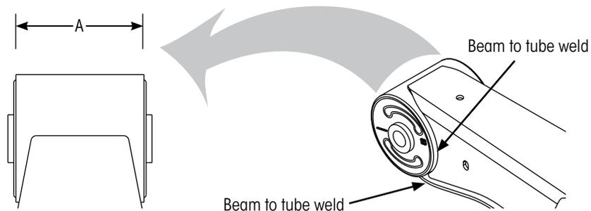
Figure 10: Bushing tube width and beam to tube weld
