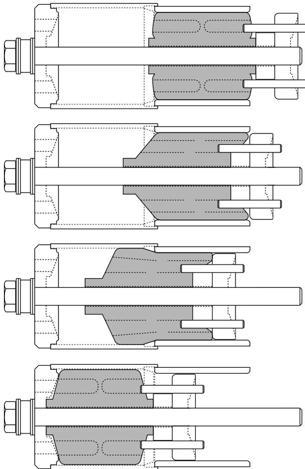
Figure 26: Typical bushing removal progression as hex head bolt is turned clockwise
