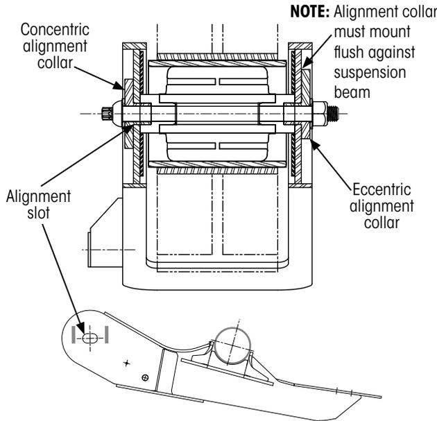
Figure 50: Y-beam QUIK-ALIGN alignment collar pivot connection
