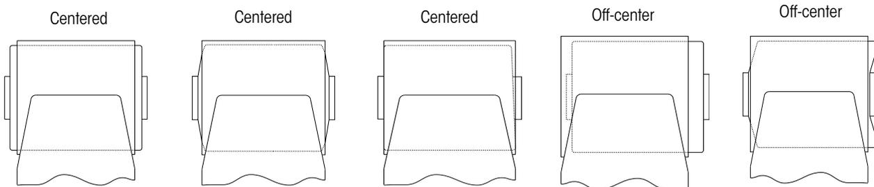
Figure 11: Bushing position relative to the bushing tube (not representative of every possible case)
