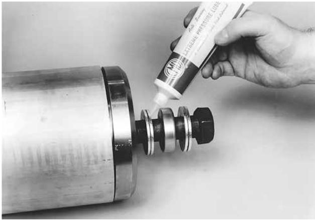
Figure 18: Applying lube to thrust washers
