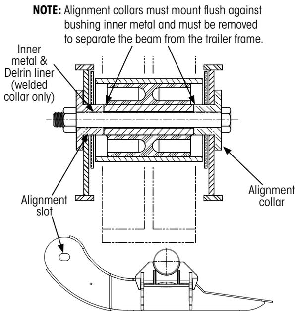
Figure 51: Y-beam Welded alignment collar pivot connection
