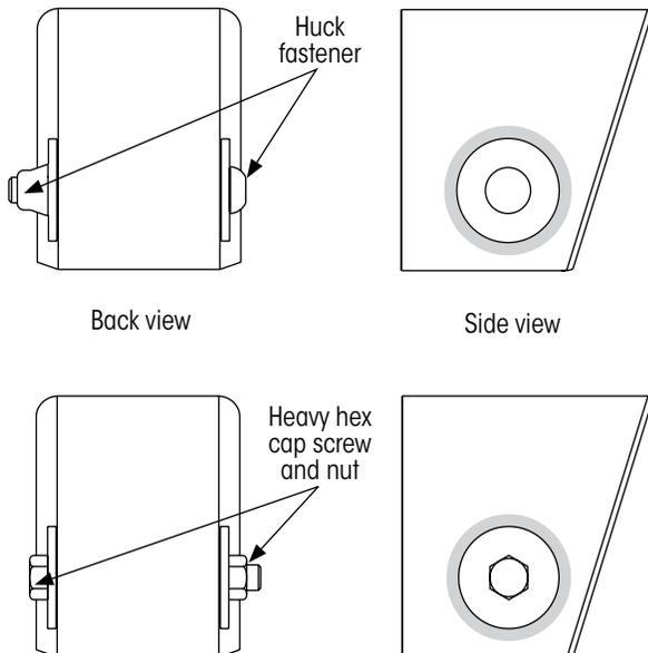
Figure 6: Welded collar style pivot connection types
