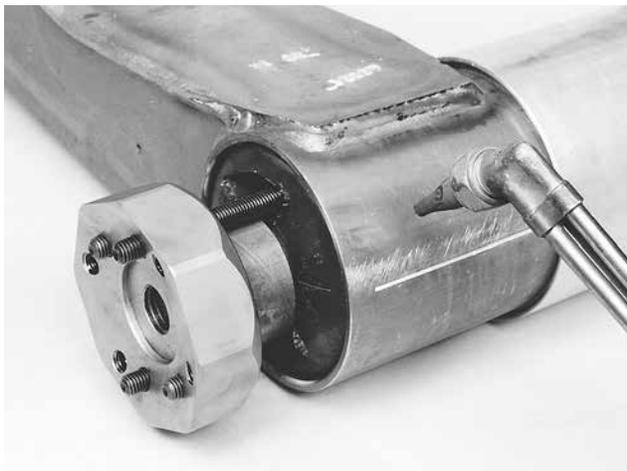
Figure 27: As a last resort, apply heat to the bushing tube
