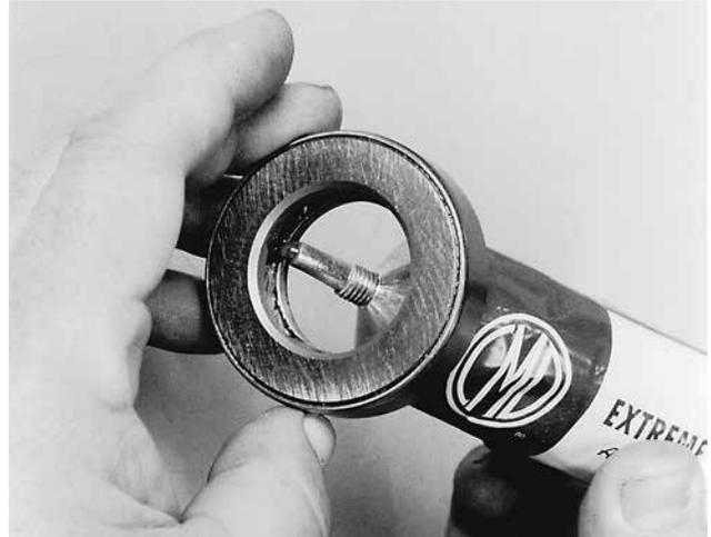
Figure 32: Applying lube to thrust bearing
