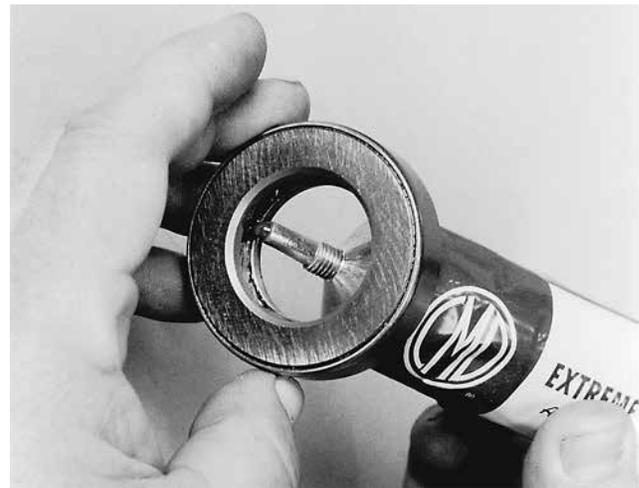
Figure 16: Applying lube to the thrust bearing
