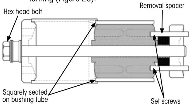
Figure 23: Wide Bushing removal
