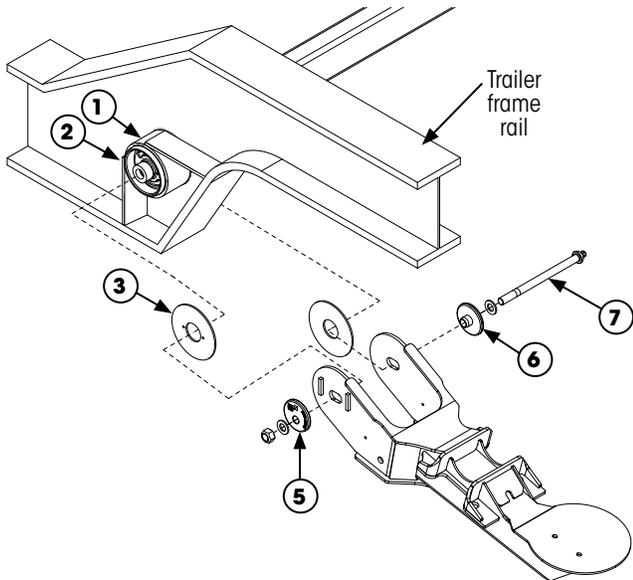
Figure 48: QUIK-ALIGN® pivot connection hardware
