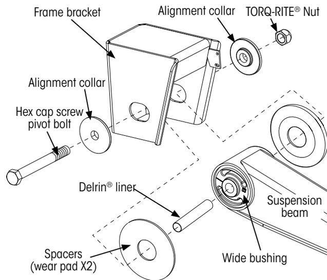
Figure 7: Welded collar style pivot connection hardware
