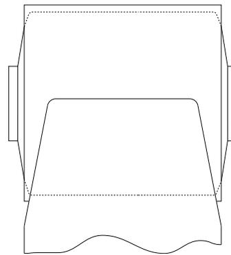
Figure 47: Bushing inner metal centered in bushing tube
