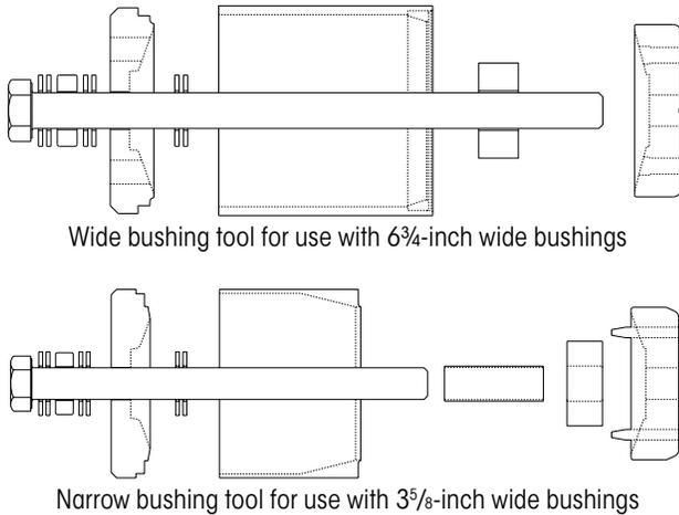
Wide bushing tool for use with 6<sup>3</sup>/<sub>4</sub>-inch wide bushings
