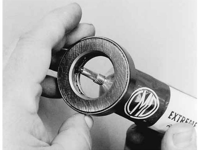
Figure 32: Applying lube to thrust bearing
