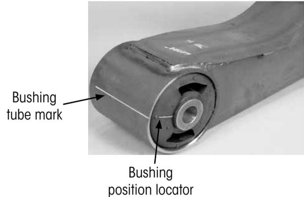
Figure 14: Properly marked bushing orientation
