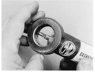
Figure 32: Applying lube to thrust bearing
