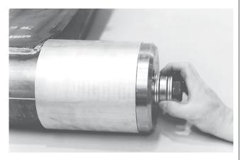
Figure 25: Ensure thrust bearing is free to turn
