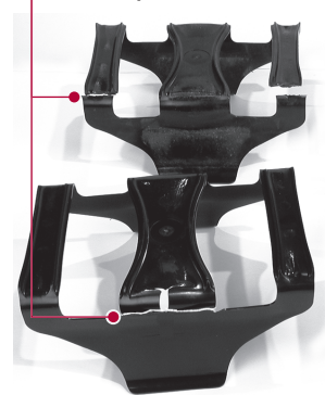
Axle Wrap Liners Cracks
