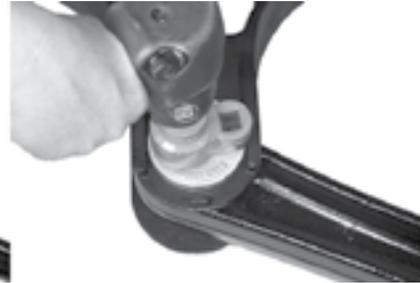
11. Once the correct axle alignment is achieved, use a calibrated torque wrench to tighten the 1" QUIK-ALIGN locknuts to  $550 \pm 25$  foot pounds torque.
