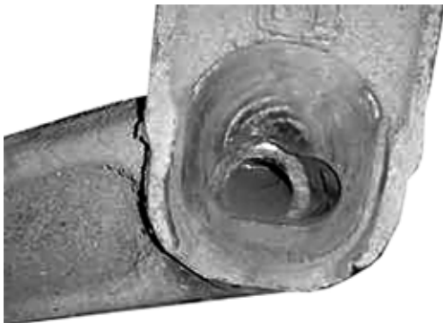
Figure 15: Hanger Damage Due to Loose Joint
