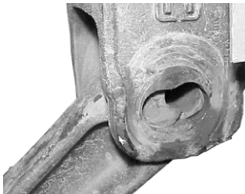
Figure 14: Hanger Damage Due to Loose Joint
