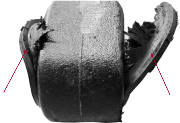
Figure 11: Disconnected Rubber Flange
