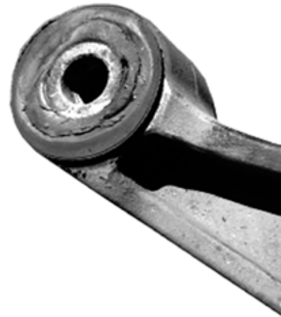
Figure 16: Pivot Bush Damage Due to Loose Joint
