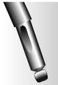
Bent or dented shock absorber
