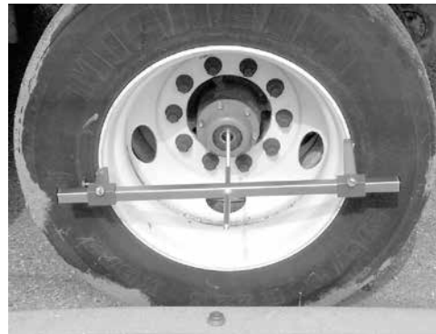
Figure 19: Installed wheel-end extender
