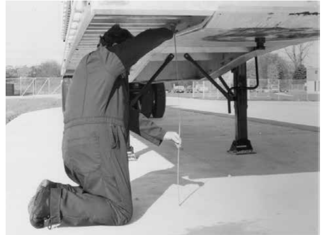
Figure 15: Measuring actual kingpin height
