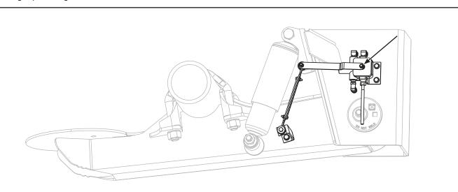
**NOTICE**: The HCV assembly (Part no. 98603-022) includes the lever arm. The nut that retains the lever arm to the HCV shaft is held tight with thread lock and MUST NOT be removed! (Refer arrows.) Attempting to remove the nut will most likely result in fracture of the HCV shaft.
