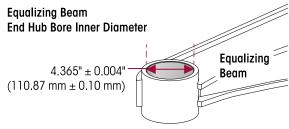
components are **NOT** within the specified range, replacement is required.
