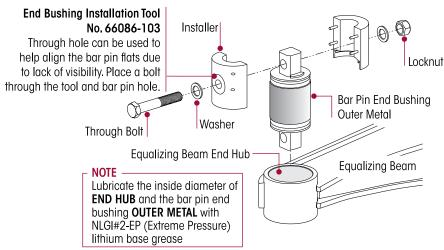
Install Hendrickson Part No. 66086-103 (OTC 1757) end bushing installation tool (refer to Special Tools Section of this publication) on the new end bushing as shown in Figure 8-43.
