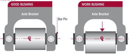
A GOOD bushing will appear centered the centerline of the bar pin in the axle bracket and equalizing beam end hub A **WORN** bushing will appear offset/below the centerline of the bar pin in the axle bracket and equalizing beam end hub
