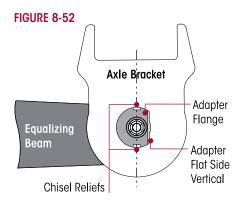
METALS CAN EXPERIENCE EXCESSIVE WEAR AND/OR FAILURE. THIS CAN CAUSE SEPARATION OF COMPONENTS AND ADVERSE VEHICLE HANDLING, PROPERTY DAMAGE OR PERSONAL INJURY.
