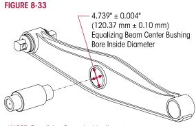
NOTE: Equalizing Beam inside diameter: Take any two readings at 90° in the same plane
