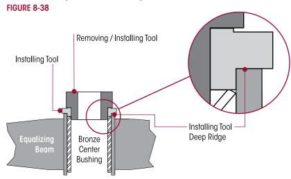
8. Using a shop press, push directly on the removing/installing tool and press in the new center bushing until the outer metal sleeve is centered and recessed in the equalizing beam's bore, see Figure 8-38.
