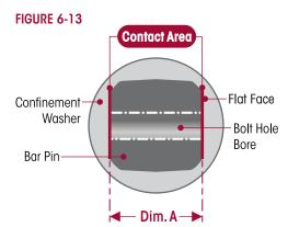
**Dim. A** - replacement is required if, bar pin measurement is less than:
