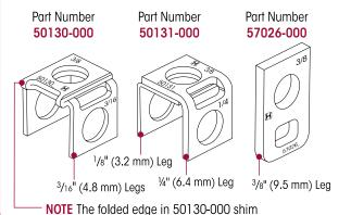
must be positioned away from bushing
