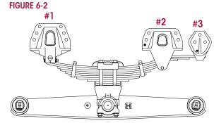
which con be caused by worn spring eye bushings. Excessive wear at either point requires hanger replacement.
