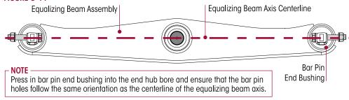
5. Verify the end bushing's outer metal is square with the end hub. Damage to the equalizing beam and the end bushing will result if the bushings are pressed in at an angle.
