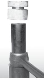
support the torque rod hub on the receiving tool with the tapered stud pointing down and the end hub centered on the tool. Be sure the torque rod is squarely supported on the press bed for safety.
