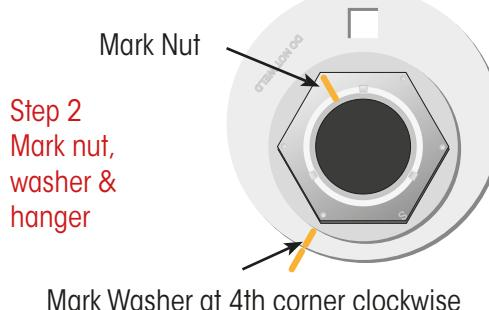
**3/** Tighten the nut **2/3** of a turn (**240 degrees**) until the marks align. Check the marks on the QUIK-ALIGN washer and hanger to ensure that the eccentric washer has not moved. **Refer Diagram.**
