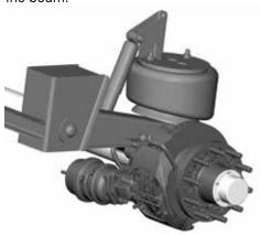
C. For low-ride / underslung air suspensions with brake chamber to the FRONT of the axle and above the beam.
