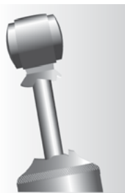
Damaged dust cover and / or shock body
