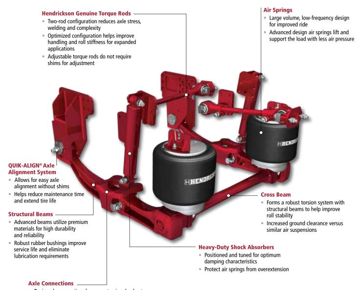
D-pin axle connection decreases torsional axle stress for reduced maintenance and increased joint integrity
