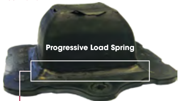
Polished Appearance — Creases formed by the folding of the rubber surface under load are acceptable.
