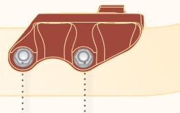
· · · · Integrated Axle Spring Seat with through bolts
