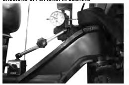
4. Checking the lower kingpin bushing
