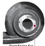
Front Spring Eye Loose Joint Worn bushing Inner Metal due to low clamp load
