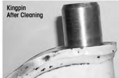
2. Inspect the kingpin for wear or damage. Use a micrometer and measure the upper and lower kingpin in two locations. Positions must be 90° opposed from each other. If the kingpin has less than 1.802" diameter, replacement of the axle is necessary, see Figures 9-54 through 9-57.
