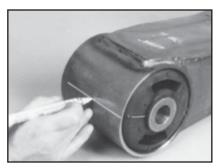
Scribe the bushing orientation on the beam tube and transition tube.
