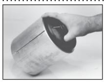
Liberally lubricate (A-14011) and push the bushing into INSTALLATION the transition tube aligning the indicator marks.
