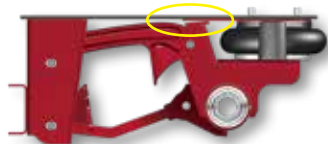
Under extreme load, secondary bump stop engages
