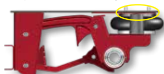
Figure A: Primary (airbag) bump stop engages
