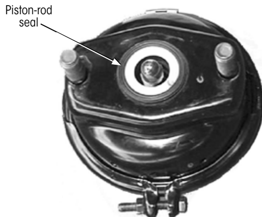
Figure 49: Brake chamber piston-rod seal
