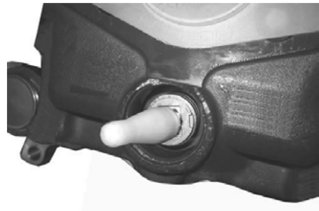
B. Placing mounting cap over adjuster
