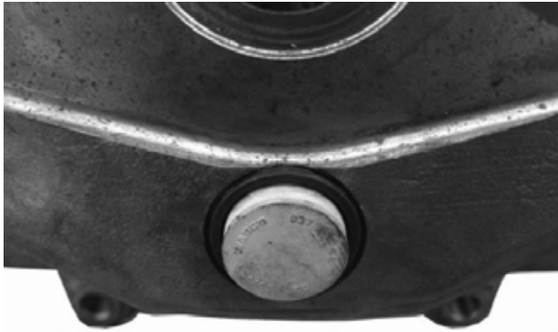
Figure 92: Adjuster plug properly inserted
