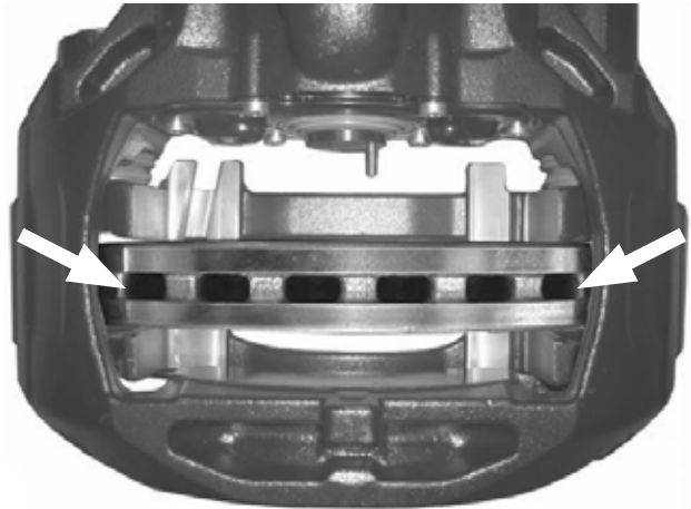
Figure 44: Positioning caliper over brake rotor
