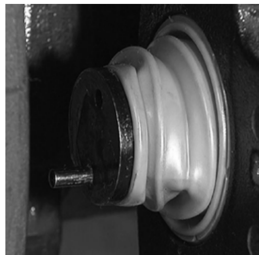
Figure 32: Wrinkled adjuster piston boot
