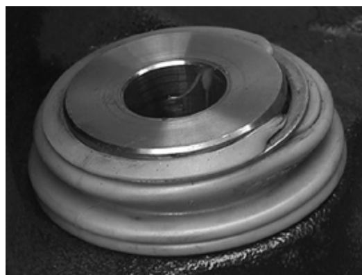
Figure 66: Improper seating of guide pin boot on guide pin
