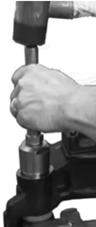
Figure 74: Using tool to install guide pin cap
