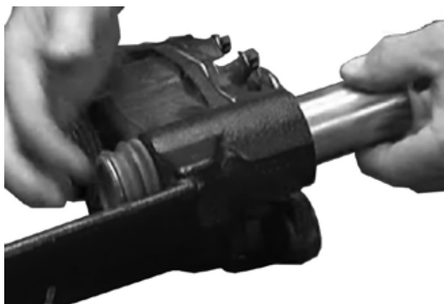
Figure 63: Inserting guide pin
