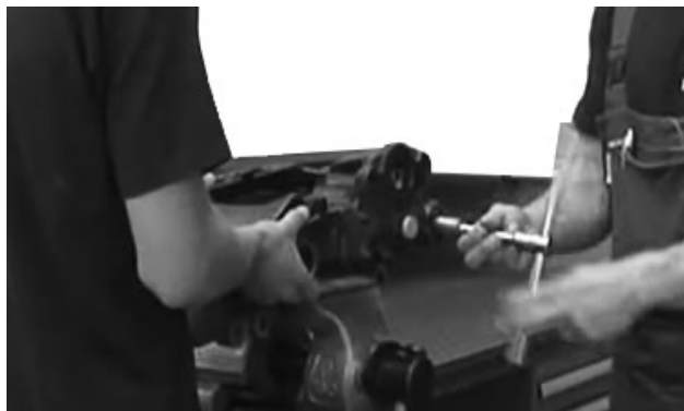
Figure 54: Supporting caliper while removing screws
