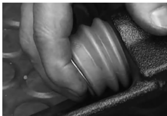
Figure 64: Seating of guide pin boot on guide pin
