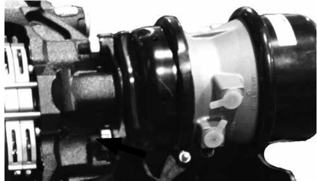
Figure 50: Installing brake chamber
