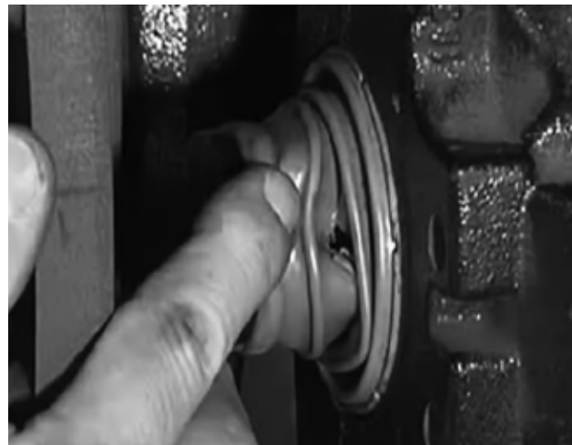
Figure 31: Adjuster piston boot damage
