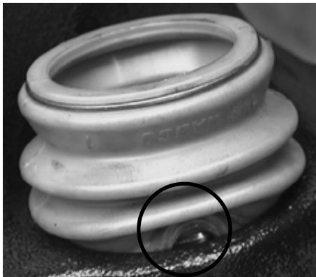
Figure 29: Improperly seated guide pin boot
