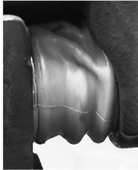
Figure 30: Twisted guide pin boot
