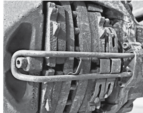
Figure 9: Broken and missing pad springs
