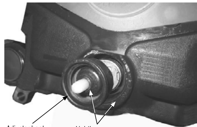
Figure 87: Installing adjuster boot
