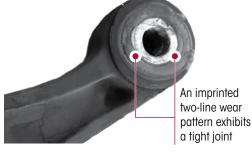
imprinted two-line wear pattern on the bushing inner metal indicates the pivot bushing is securely clamped in the frame hanger.
