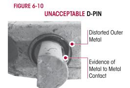
D-pin bushing replacement IS REQUIRED when:
