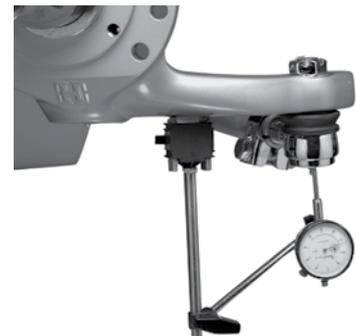
11. Position yourself directly below the tie rod end. Using both hands, grab the assembly end as close to the tie rod end as possible (no more than 6" or 152.4 mm). Apply hand pressure with reasonable human effort vertically up and down in a push-pull motion several times (using approximately 50 to 100 pounds of force). Check for any movement or looseness at both tie rod end locations (See Figure 9-4).
