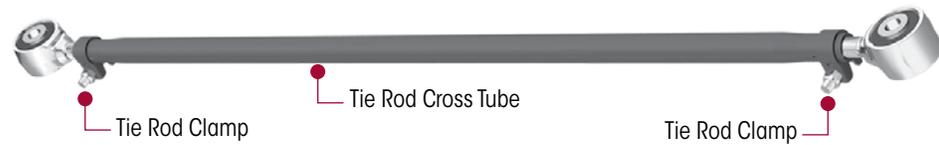
2. Rotate the cross tube to achieve the recommended  $\frac{1}{16}$ " to  $\frac{1}{8}$ " toe-in specification.
