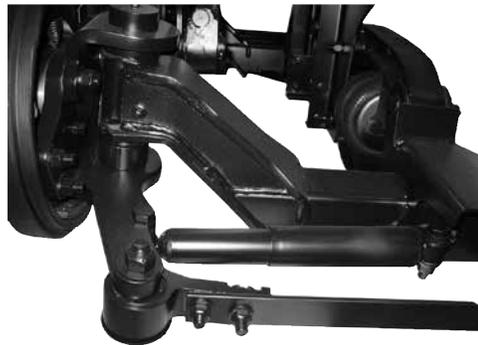
7. Remove the bolts that connect upper kingpin assembly to the steering knuckle.
