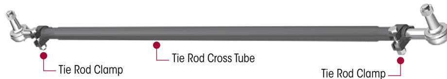
1. After the inspection, if a toe adjustment is necessary, loosen the tie rod clamp fasteners on both ends (see Figure 9-11 above).
