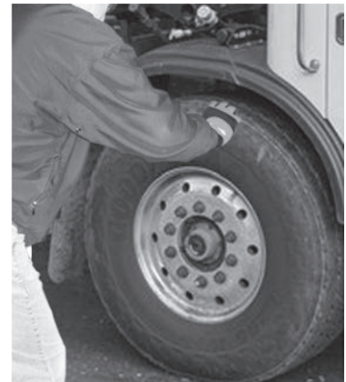
FIGURE 7-16 Move TOP and BOTTOM of the tire in and out
