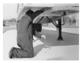
Figure 5: Measure from ground to kingpin
