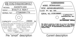
Figure 11: Typical suspension ID tag on INTRAAX suspensions
