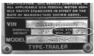
Figure 4: Sample trailer VIN plate
