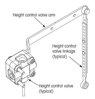
Figure 13: Typical height control valve components
